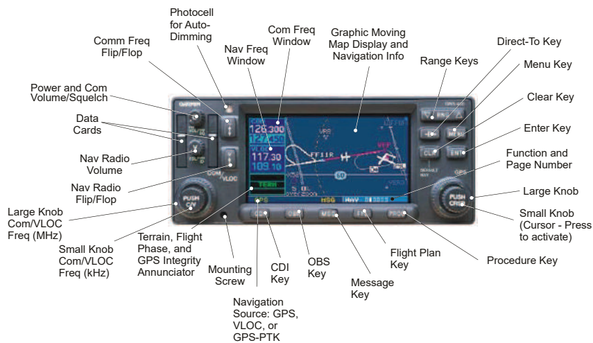
Figure 1 - 430W Series Control and Display Layout
